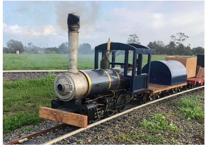
Declan Henry's 0-6-0 carves its way through the wyes while sporting its new pilot beam.
