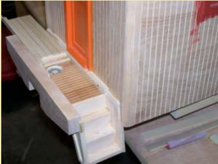
The grated porch floor is removable to get to the coupler pin.
