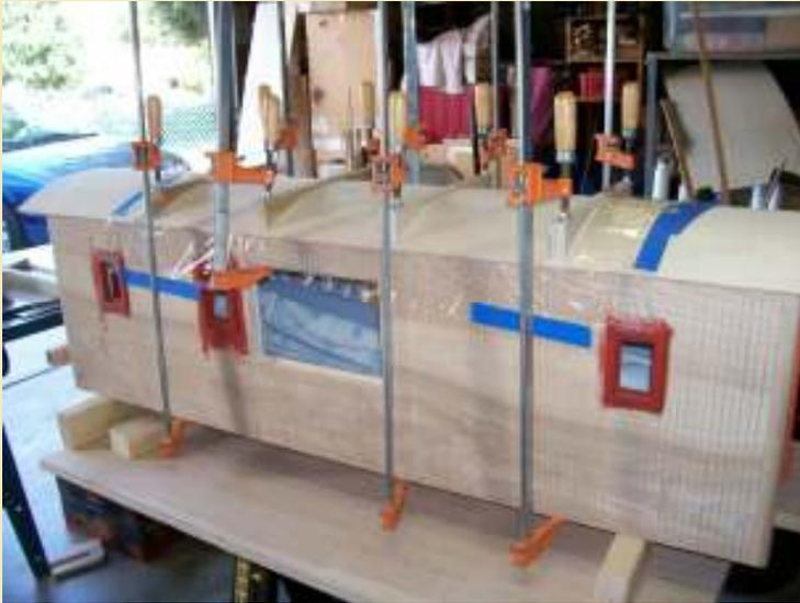
Never have enough clamps. Cellophane used to prevent glue from oozing onto structure.
